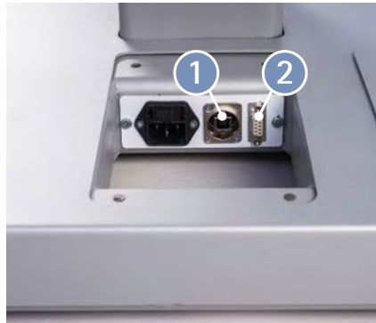
Figure 4 – 11: Connection for ECG recorder/PC ECG system
