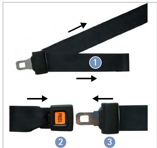
Figure 12-5: Adjusting and closing the safety belt
