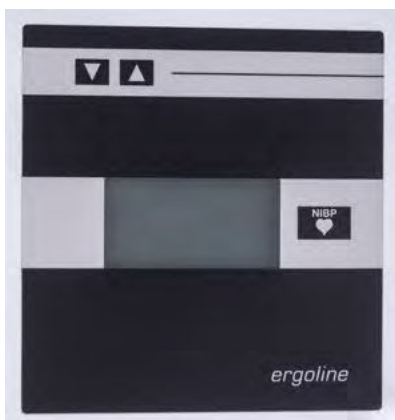
Figure 8-1: Control terminal D (Service) (installed under the couch surface – standard)
