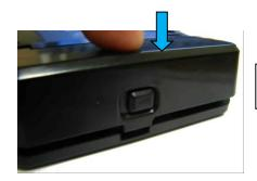
As indicated in the illustration, close battery compartment cover and press on it until latches into the base part.
