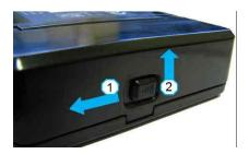
Open battery compartment cover by moving Left and Up the battery compartment cover latch.
