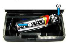
Insert a fresh AA battery as indicated in illustration, be sure to first insert from the negative terminal. Pay special attention to the correct polarity of the battery
